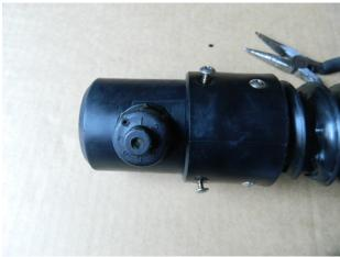
2. Detach the nozzle but do not pull it free yet - the solution tube is still attached!
