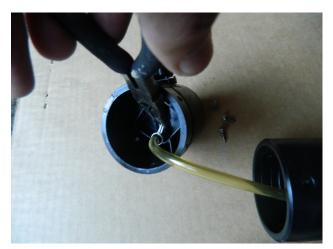
4. Pull the solution tube free from the nozzle.
