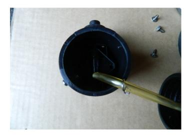
5. Remove the 3 screws closer to the machine body (leave the other 3 screws alone).
