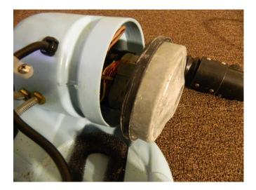
d. Unplug the wires from the motor.
