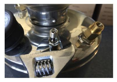
2.3. With a strong force, **push** the valve into the tank and retrieve it from the tank.
