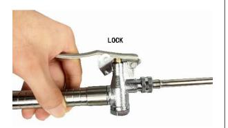
**To stop automatic-spray:** Hold trigger, then either unlock using your finger, or quickly point the handle up.
