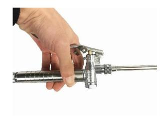
8. **Start spraying** by squeezing the trigger.
