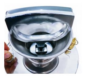
2. **Pull out cylinder.** Turn the handle counter-clockwise (without pushing in) until it comes loose, then pull out.
